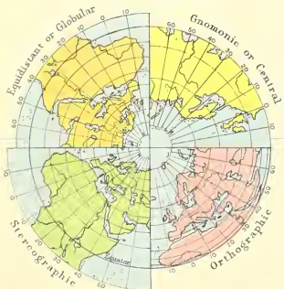
The Gnomonic Projection cannot be made to include the whole hemisphere. The Stereographic and Globular Projections can be extended to include more than the hemisphere.
